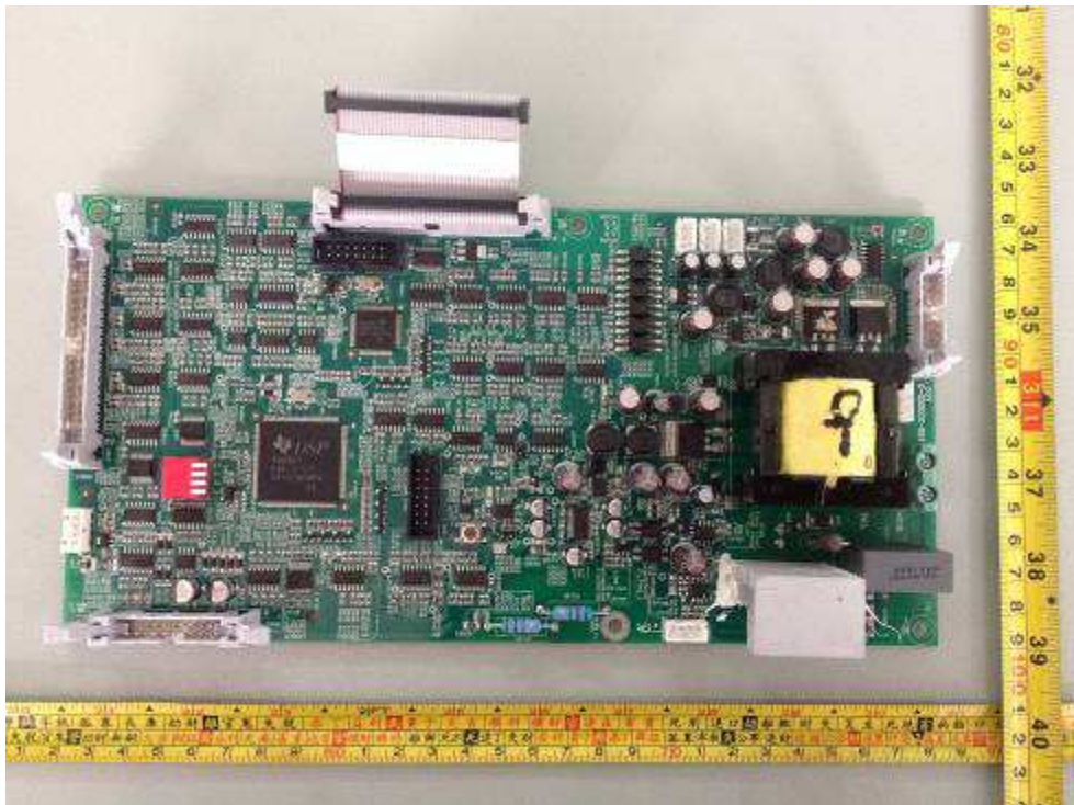
Front view of the control board
